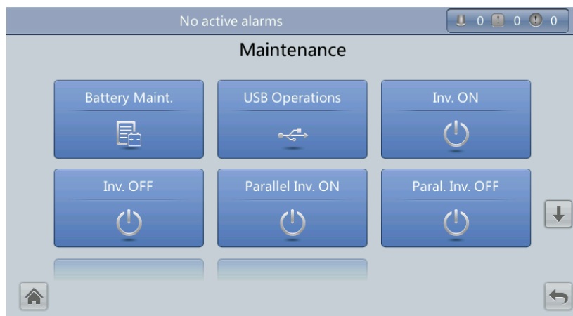
Figure 4-53 Maintenance Screen (parallel system)
