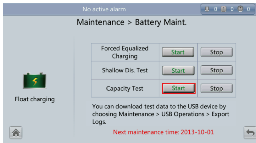
Figure 5-25 Starting a capacity test
