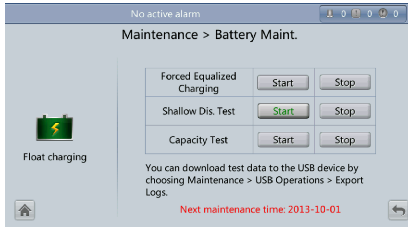
Figure 5-24 Starting a shallow discharge test
