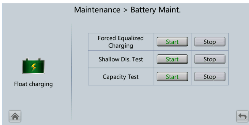
Figure 4-38 Battery Maint. (lead-acid battery)
