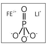
Similarly to lead acid batteries, li-ion uses a positive cathode, a negative anode and an electrolyte as a conductor. The key difference being the chemical characteristics found within them. Lithiumion cathodes are metal oxide based and the anodes carbon based. VRLA batteries use lead dioxide cathodes and lead anodes. It is these differing chemical compositions of the anode and cathode materials that determine the overall performance of the battery.
