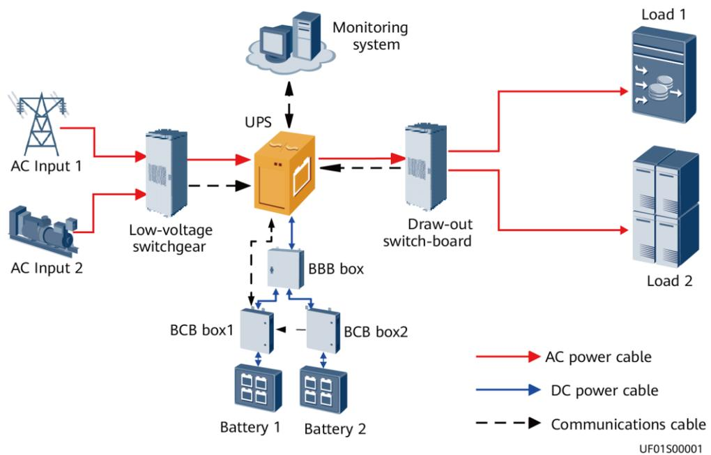
**Figure 3-2** Typical application scenario of 1+1 parallel system
