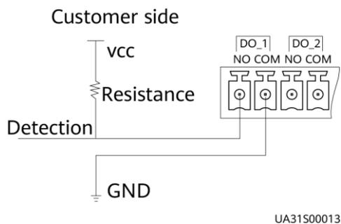
**Figure 4-11** Wiring method 2
