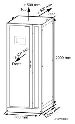
Figure 6-1 UPS installation clearances (400-600 kVA)
