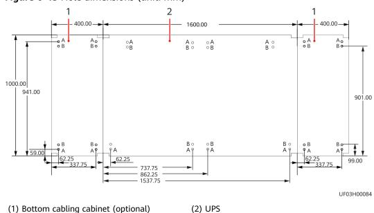
Figure 6-43 Hole dimensions (unit: mm)
