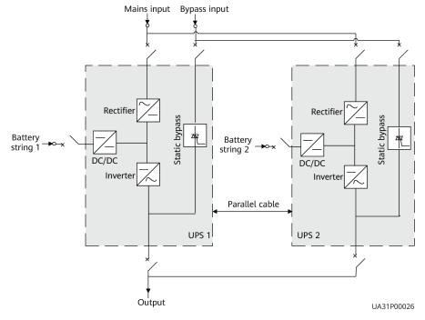
Figure 6-57 Conceptual diagram of a 1+1 parallel system
