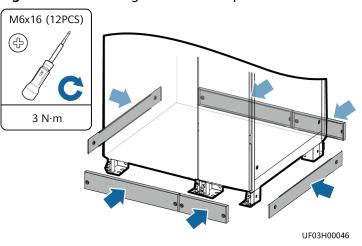
Figure 6-22 Installing anchor baffle plates
