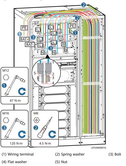
Step 4 Connect signal cables. Bind cables to the cabinet nearby.
