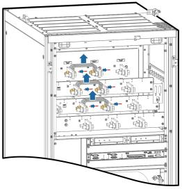
Figure 6-27 Installing cables
