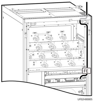
Figure 6-16 Installing a signal cable
