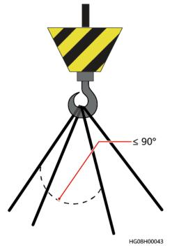
• Do not drag steel ropes and hoisting tools or bump hoisted objects against hard objects during hoisting.
