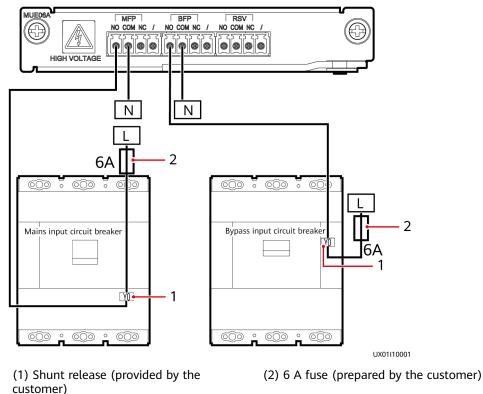
**Figure 6-60** Cable connections between the backfeed protection card and shunt release
