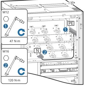
Figure A-1 Short-circuiting the input N and PE (400–600 kVA)
