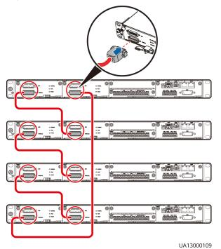
Figure 8-1 Control cable connections in a parallel system of four UPSs
