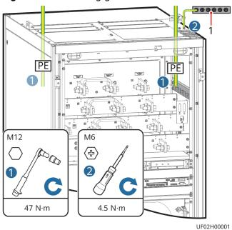
Figure 6-13 Installing ground cables
