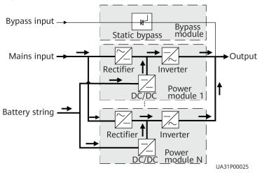
Figure 2-9 Conceptual diagram in source-share mode
