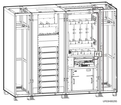
Figure 6-53 Installing a communications cable
