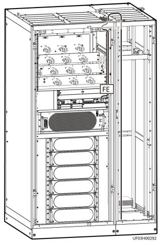
Figure 6-28 Installing a signal cable
