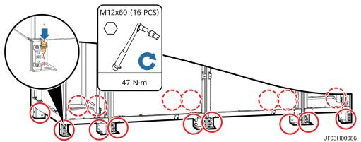
**Step 7** Install anchor baffle plates.
