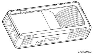
Figure 5-12 DIP switch on the ambient T/H sensor
