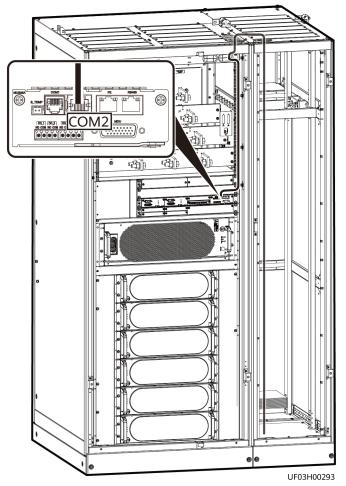
Figure 6-29 Installing the SmartLi communications cable
