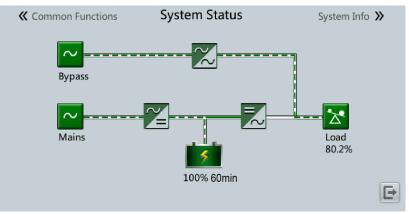
After you shut down the inverter, the UPS supplies no power if the bypass is abnormal, which causes a power failure for the loads.
