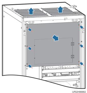
**Step 2** Remove the bottom cabling cover from the bottom cabling cabinet.
