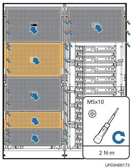
**Figure C-2** Installing copper bar protection components (800 kVA)
