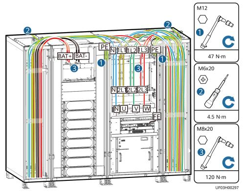
Step 4 Connect signal cables. Bind cables to the cabinet nearby.
