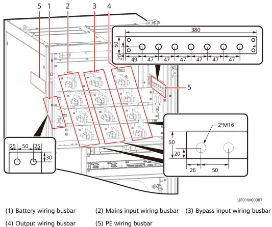
Figure 6-5 400–600 kVA cabinet copper bar layout and specifications (unit: mm)
