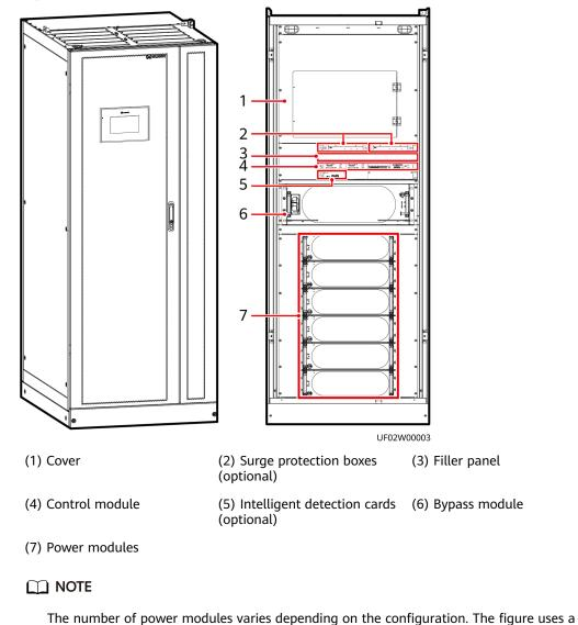
Figure 3-2 UPS exterior and interior (600 kVA)
