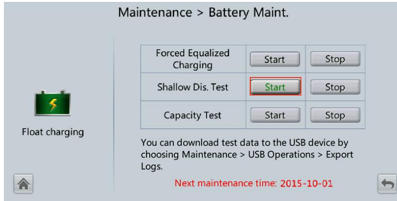
Figure 5-20 Starting a shallow discharge test
