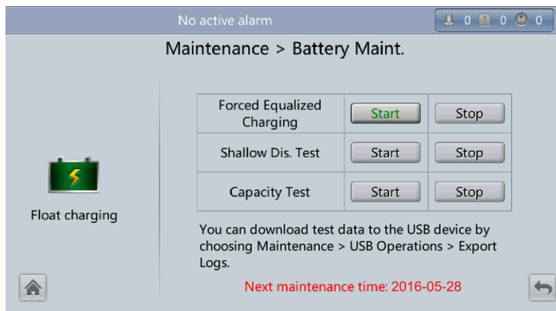
Figure 4-47 Battery Maint. screen
