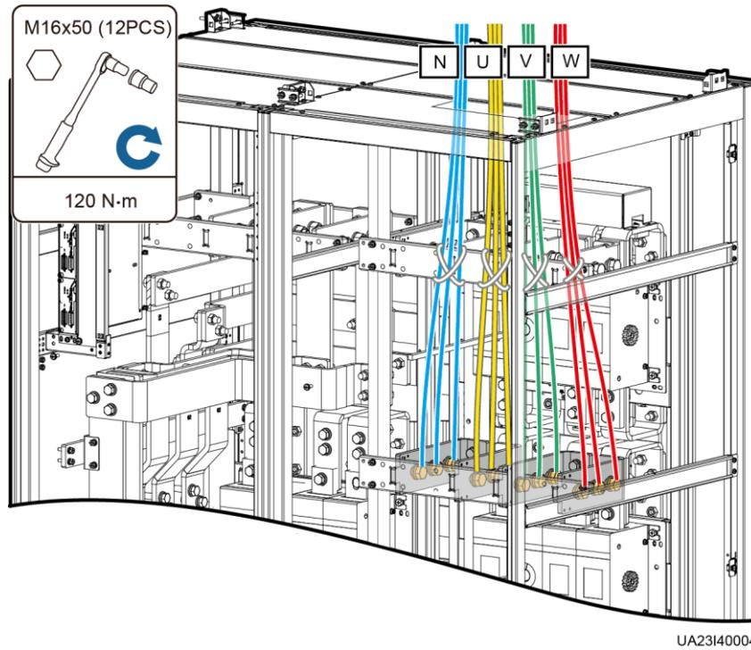
**Step 8** Connect the bypass input power cables. (Perform this step only when the mains input and bypass input use different power sources.)
