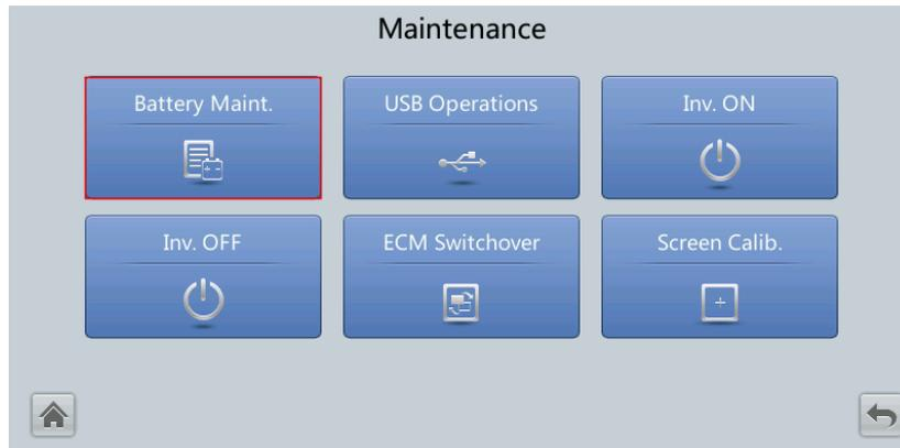
**Step 3** Tap **Start** next to **Forced Equalized Charging** to start a forced equalized charging test.
