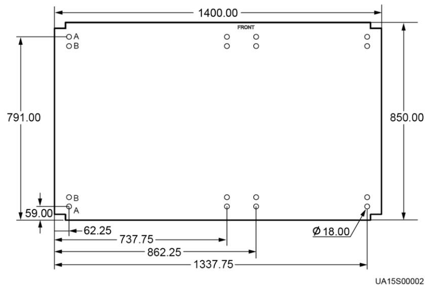
**Step 2** Use a hammer drill to drill holes for installing expansion bolts, and install expansion sleeves in the holes. [Figure 3-22](#) shows expansion bolt composition. [Figure 3-23](#) shows how to install an expansion bolt.
