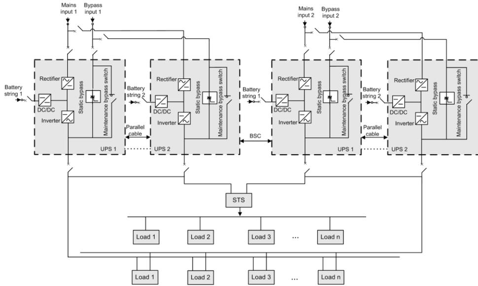
**Figure 3-101** Cable connections for a dual-bus parallel system (400 kVA UPS)
