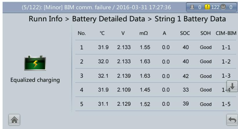
This screen displays the temperature, voltage, internal resistance, current, SOC, and SOH of a single battery in the battery string, and the mapping between the CIM and BIM.
