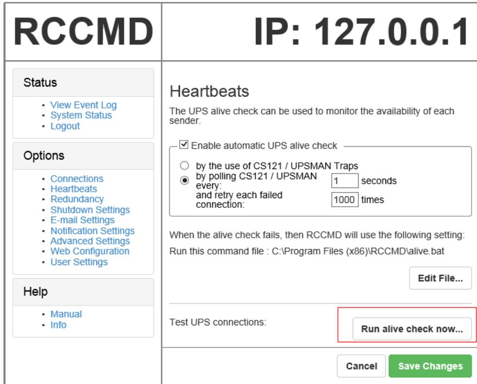
Figure 4-110 Detecting heartbeat manually and successfully
