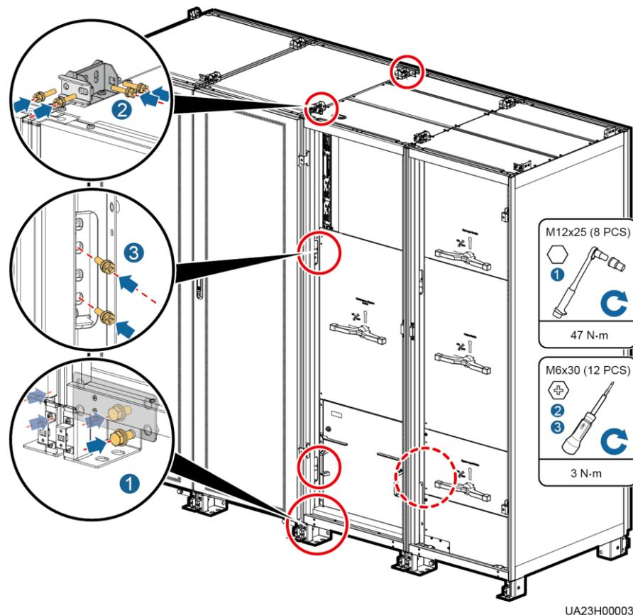
**Step 4** Use M12x60 expansion bolts to secure the cabinets to the expansion bolt holes on the ground. [Figure 3-34](#) shows how to secure the power cabinets.
