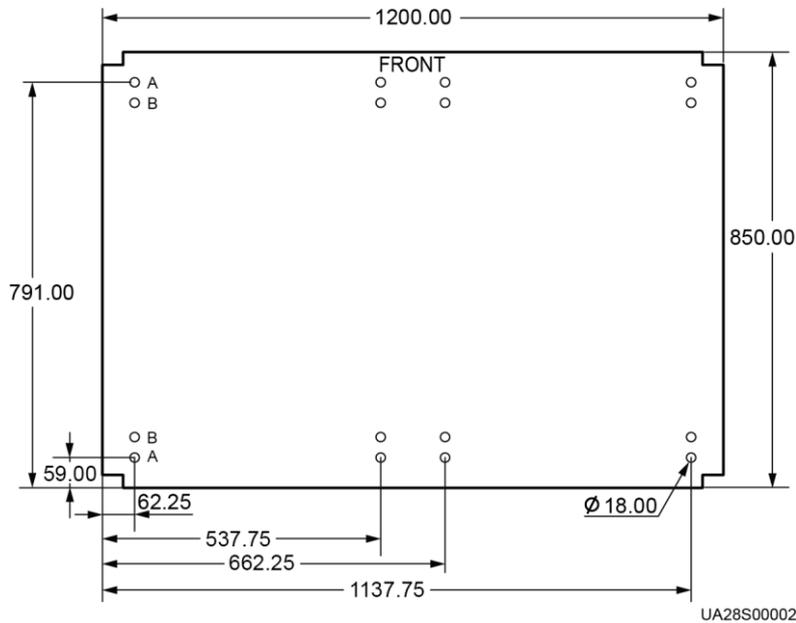
**Figure 3-21** Mounting hole dimensions for the 600 kVA UPS (unit: mm)
