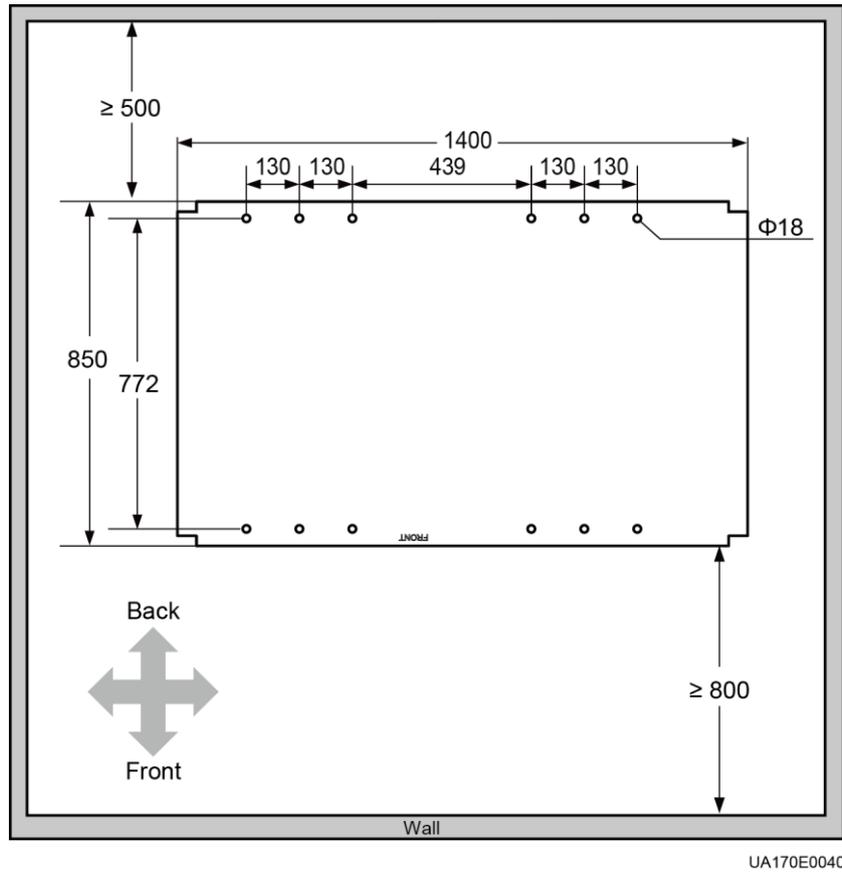
**Figure 3-45** Dimensions of antiseismic kit mounting holes for the 800 kVA UPS (unit: mm)
