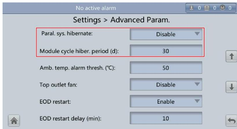
**Step 3** On the LCD, set **Paral. sys. hibernate** to **Enable**. A confirmation message is displayed, as shown in [Figure 5-38](#).
