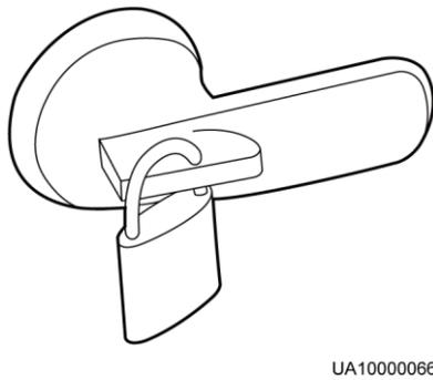
**Figure 3-27** Installing a lock for the maintenance bypass switch (600 kVA UPS)
