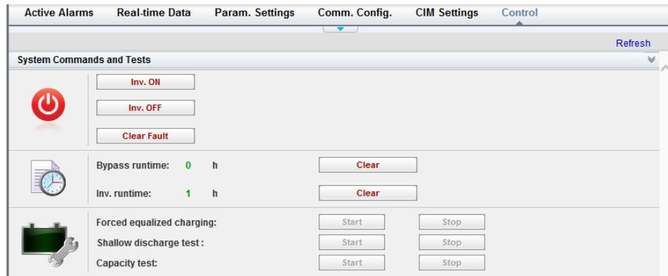
**Step 3** Check that the EPO alarm is cleared by viewing active alarms. If the system bypass input is normal, the UPS transfers to bypass mode.
