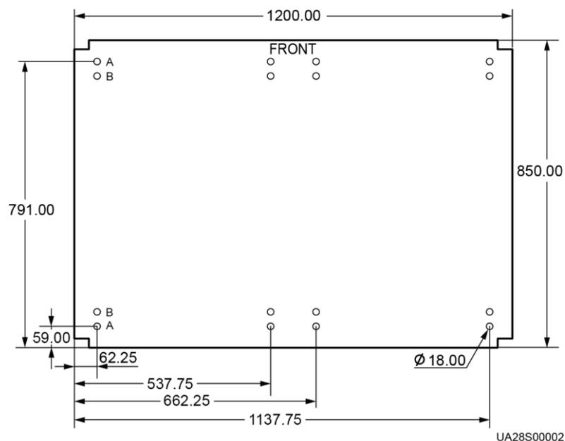
**Figure 3-29** Mounting hole dimensions for the 600 kVA UPS (unit: mm)
