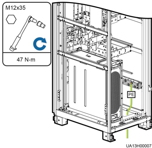
**Step 6** Connect the bypass input power cables. (Perform this step only when the mains input and bypass input use different power sources.)
