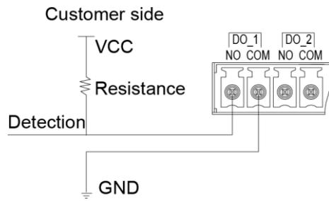
**Figure 2-28** Wiring method 2
