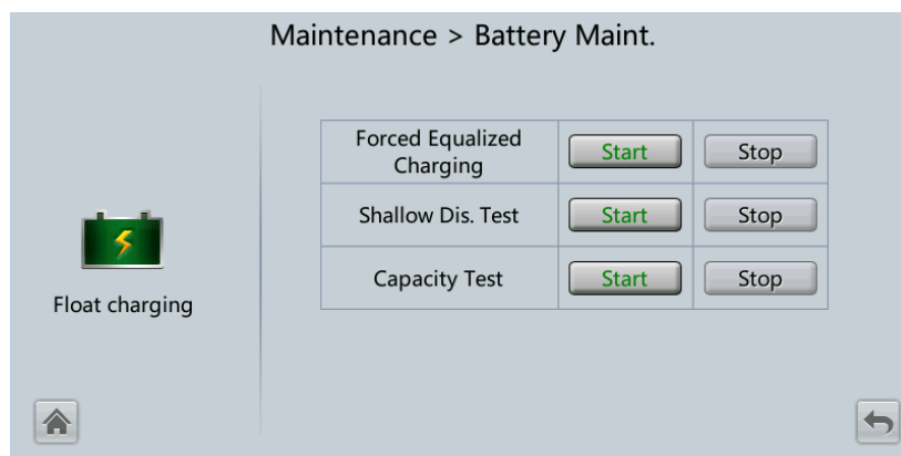
Figure 4-37 Battery Maint. screen
