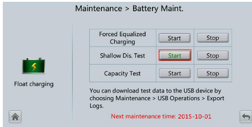
Figure 5-21 Starting a shallow discharge test
