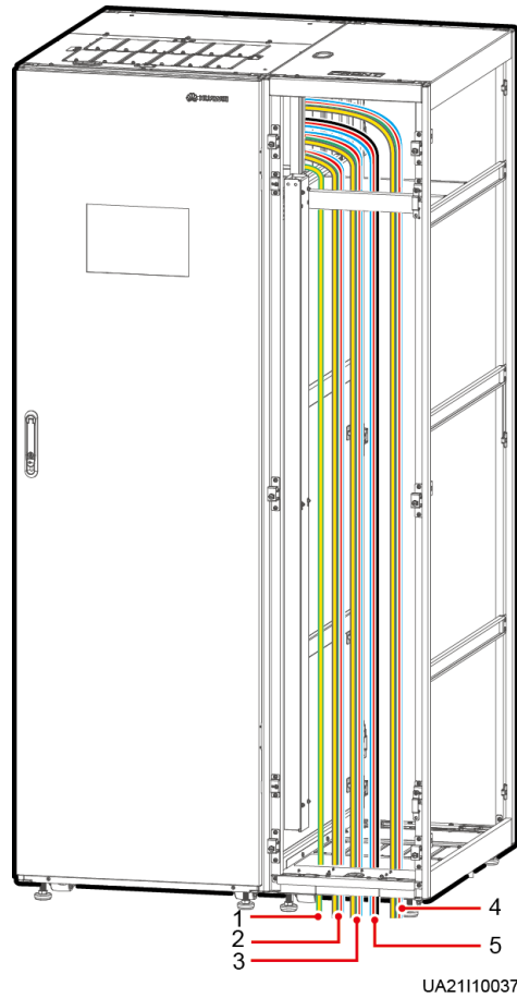
Figure 3-49 Connecting the ground cable and power cables
