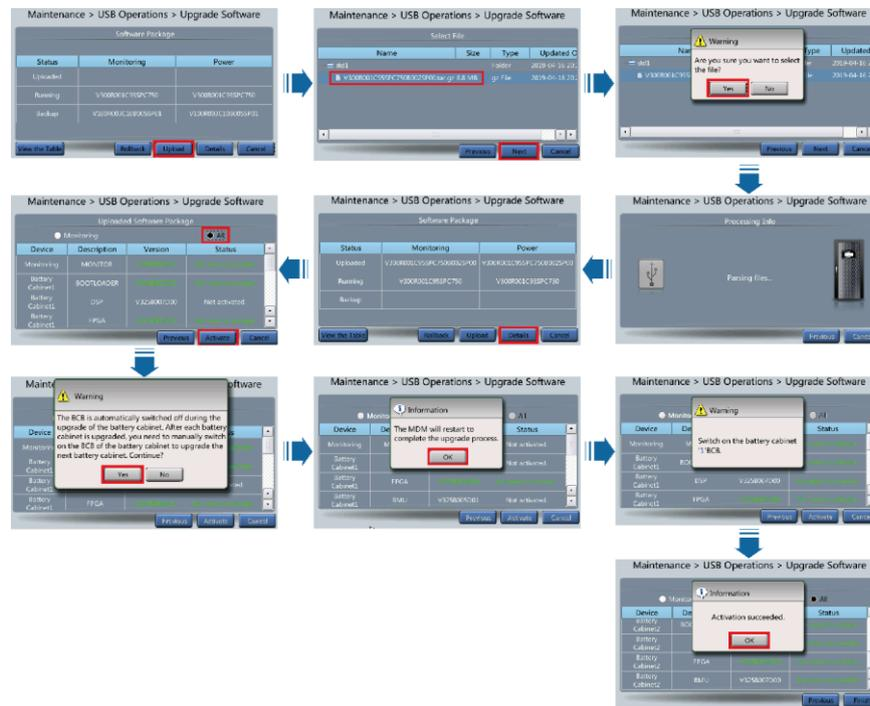
**Figure 8-4** Uploading and activating the software (the BCB switches of all battery cabinets are OFF)
