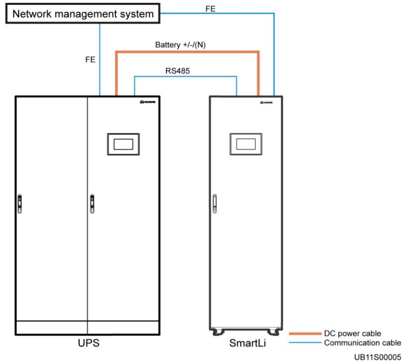
**Figure 2-2** Networking with multiple battery cabinets
