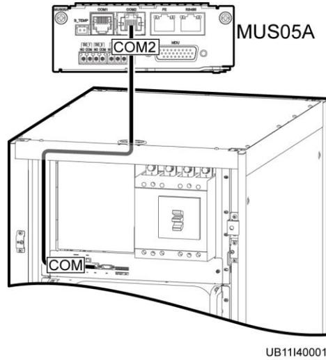
**Figure 3-31** Connecting communications cables (parallel system, for example, five cabinets)
