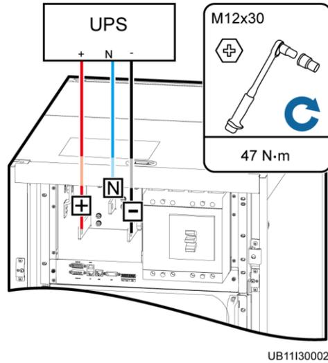
**Figure 3-29** Installing power cables (parallel system, for example, five cabinets)
