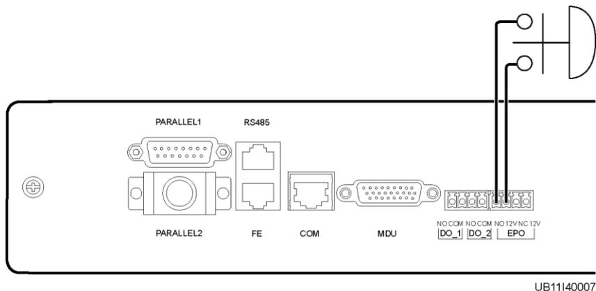
**Figure 3-26** Cable connection for an NC EPO switch
